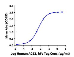
Immobilized Biotinylated SARS-COV-2 Spike S (Trimer), His Tag at  $2\mu$ g/ml (100 $\mu$ l/well) on the streptavidin precoated plate ( $5\mu$ g/ml). Dose response curve for Human ACE2, hFc Tag with the EC50 of 5.9ng/ml determined by ELISA.
